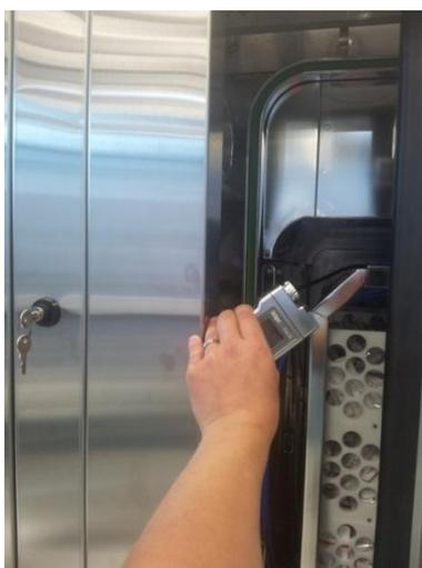
*Figure 12: Peroxide residue testing at chamber door-open, using hand-held device*
