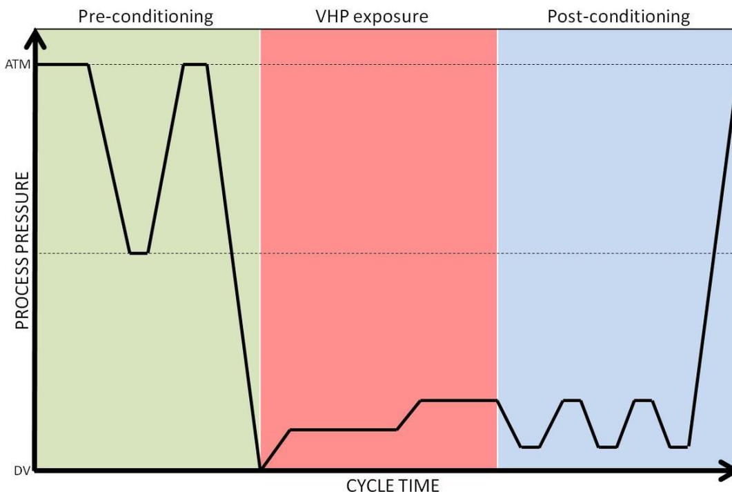
Graph 1: STERIS VHP LTS-V Surfaces Terminal Sterilization (vacuum) process steps
