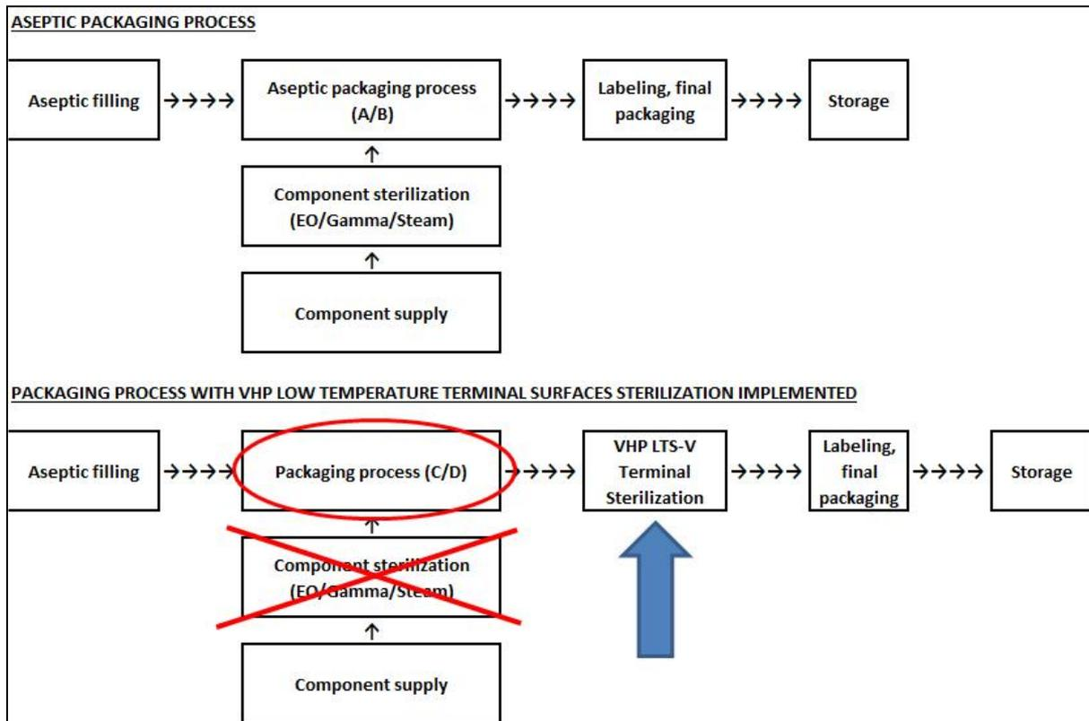
Schematic 1: Generic aseptic packaging process before and after implementing LTS-V terminal sterilization phase
