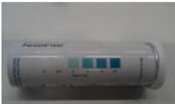
Figure 11: Quick on-site strip test for ingress testing (container integrity).
