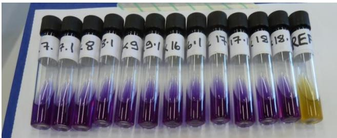
Figure 10: Biological indicators in test tubes. Control positive on the right.
