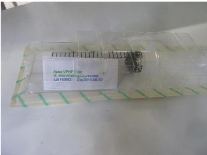
*Figure 8: Tyvek-enveloped biological indicator placement inside packaged device*
