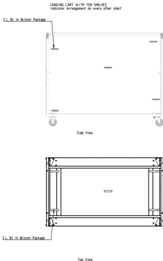
Figure 6: Typical biological indicator test map for entire load
