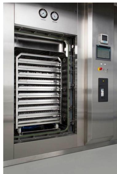
Figure 3 & 4: Loading a VHP LTS-V sterilizer.
